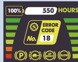
🔍 Operation status & fault diagnosis are integrated onto the tiller handle display for easy troubleshooting.
