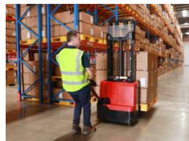
When truck is down, release the brake to move the unit manually.
