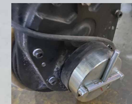
(Optional) Manual release, can avoid the use of power consumption or circuit failure, the vehicle can not move into paralysis
